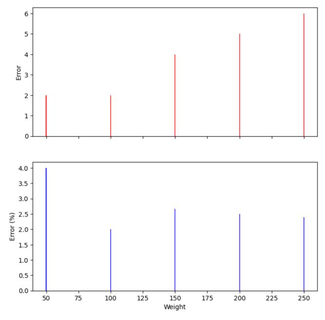
Therefore we observe an almost linear pattern in the maximum deflection along with some outliers which are quantified by the error plots. These help in quantifying the objectives of the experiment.
