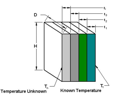
Engineer's Edge. (n.d.). Conduction through a Multilayer Isothermal Wall [Online image]. Retrieved from https://www.engineersedge.com/heat\_transfer/conduction\_multilayer\_isothermal\_wall.htm
